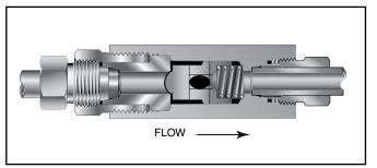
Minimum operating temperature for standard ball check valves 0°F (-17.8°C).
